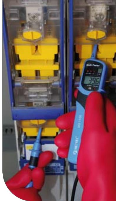
The MD 1100 is a high-quality voltage tester designed for the most demanding duties. With a broad spectrum of measurement functions and CAT IV/1000 V overvoltage category, the device is suitable for both the industrial sector and for everyday maintenance and repair practice.
